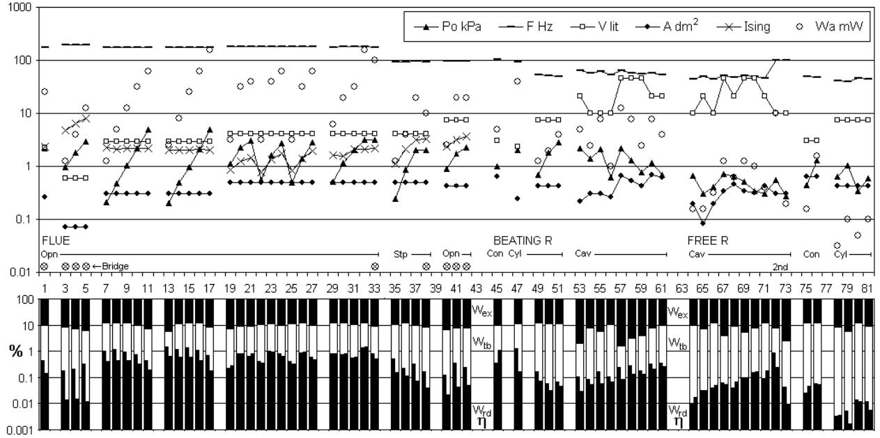
Figure 1: Top: Some dimensional data and measurements for the pipe samples. Bottom: Computed cumulative percentage of input power developed in radiated sound  $W_{rb}$ , resonator loss  $W_{ib}$ , and the excitation mechanism  $W_{ex}$ .  $W_{ra}$  corresponds to efficiency  $\eta$  and is split into a left bar for the result found from external sound, and a right from internal sound pressure.
