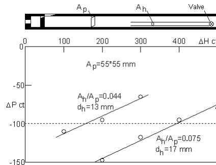
Figure 7: Narrow tube detuner and measured effect.
