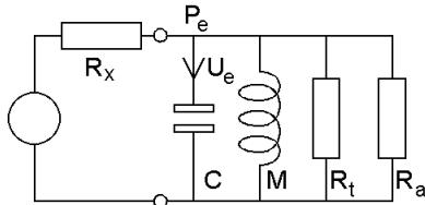
Figure 3: A resonator modeled as a single RMC parallel circuit, with resonance angular frequency  $\omega = (MC)^{1/2}$  and quality factor  $Q = R/(\omega M) = \omega C/R$ , where R is the parallel combination of exciter, turbulence and acoustic components.
